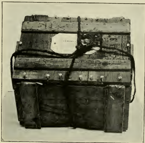
Fig. 45. Box showing thoughtlessness of an exhibitor using fifteen screws instead of hinges and one screw.
