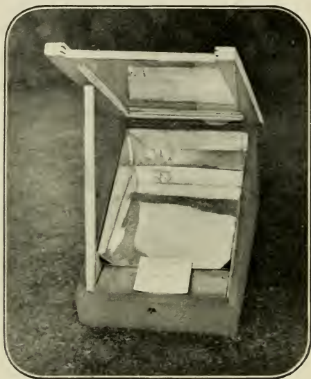
Fig. 41. Mr. G. W. Judge's Home-made Solar Wax Extractor.
